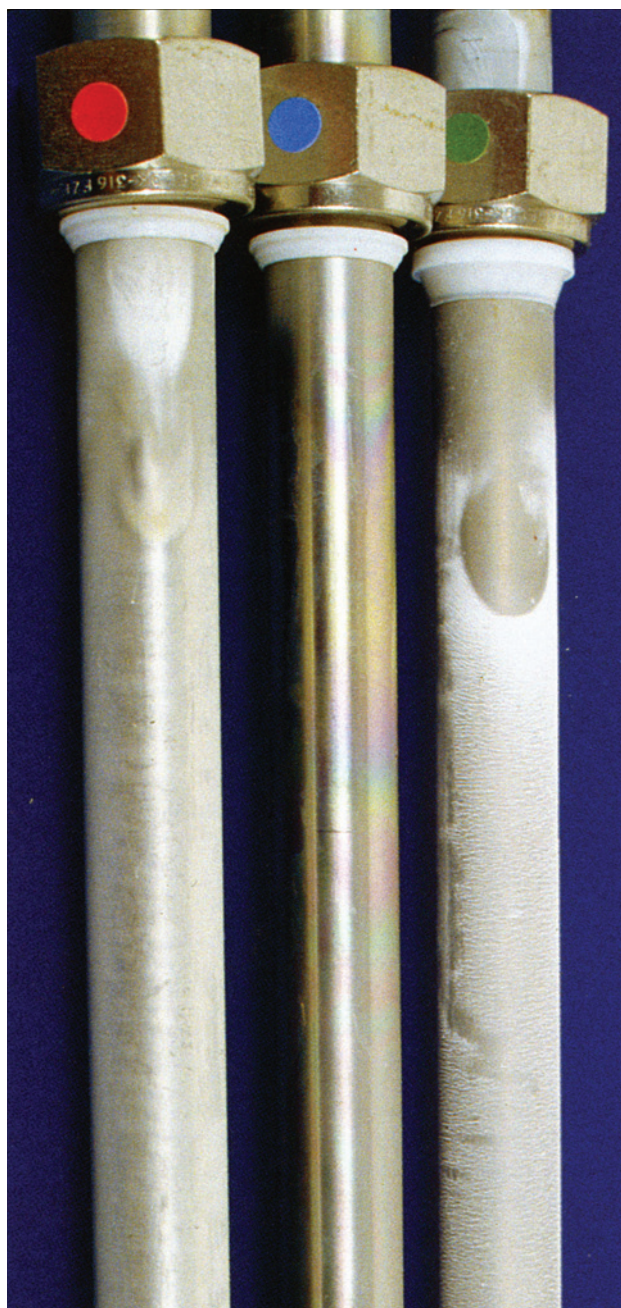
Photo 4: Heat Exchanger Rods ● AA:AMPS ● Versaflex ONE ● Polymaleic Acid
